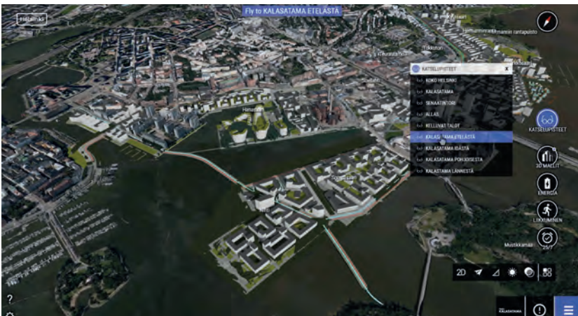
▲ For the Helsinki 3D+ project, reality modelling plays a vital role, enabling the government to deliver the reality mesh and generate a 3D semantic information model in CityGML format to city stakeholders for developing projects, as well as to citizens, companies, universities, and researchers. (Image courtesy of City of Helsinki)
