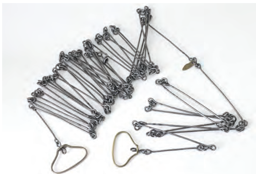
▲ Surveyors in the colonial period measured distances using chains. The favoured form was the Gunter, introduced by the English mathematician Edmund Gunter in 1620. (Courtesy: National Museum of American History)
