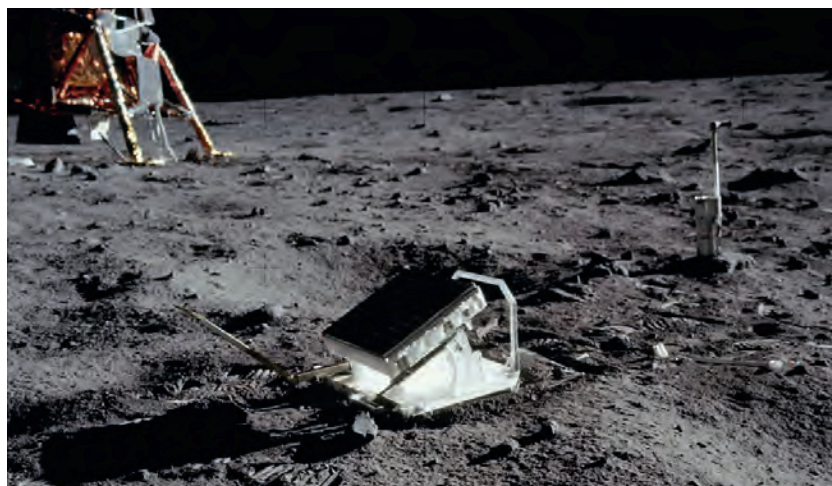
▲ A retroreflector left on the moon by astronauts on the Apollo 11 mission. The Lunar Laser Ranging experiment, which is still ongoing, measures the distance between surfaces of Earth and the moon.
