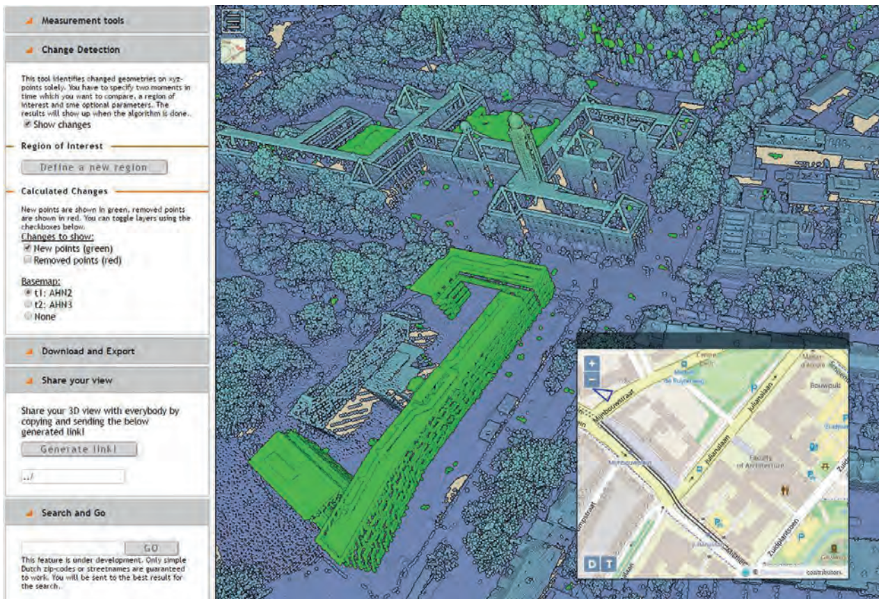
▲ Change detection in Dutch Point Cloud Height Model AHN2-AHN3 – MSc Geomatics student project, TU Delft.
